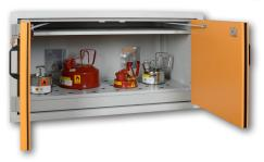
Store LAB (Type 30) with Fire Resistance >30 minutes Flammable/Corrosive/Acid/Toxic/Pesticide Cabinet, 12 Gallon, 45 Litre, Self Closing, 2 Doors, 1 Shelf, Grey Body RAL7035, Daffodil Yellow Door RAL1007, Levering Feet, Auto Thermal Closing Mechanism, Height-adjustable shelves at intervals of 32 mm, Levering Feet for levelling, With Base Sump Tray and Perforated Cover Plate at Base, Cylinder Lock on Doors, Door Hinge to Right. Markings according to DIN EN 14470-1 / TRGS 510 / ISO 3864 / ASR A1.3
